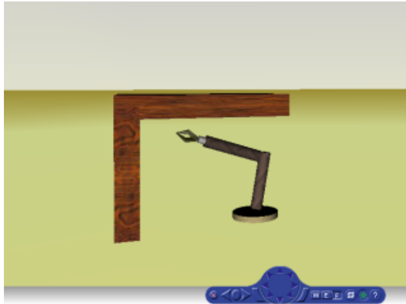
Figure 7. 2-DOF revolute joint robot in VR
