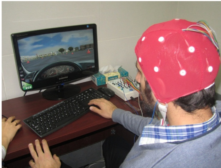
Figure 2 Experimental task, one of participants during driving at 3D-driving school simulator.
