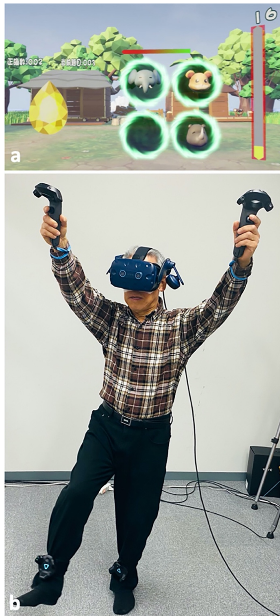
Figure 1. (a) The interface of our motion video game in the virtual reality (VR) environment. (b) An older player wears sensors while playing our game. Body parts are mapped to the position of the corresponding “Whac-A-Mole” hole.
